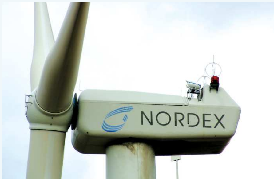
The Vindicator Laser Wind Sensor is being tested to provide wind turbine control based on wind ahead of the turbine blade. (Photo courtesy of OADS.)
