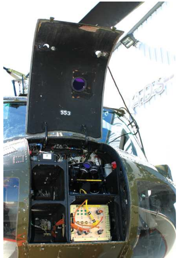
A close-up of OADS LIDAR sensors. (Photo by the author.)
